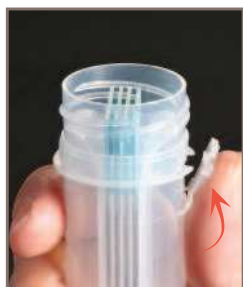
Push up the attached tab on side of vial.
